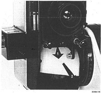
6. Swivel the assembled instrument out of the Styropor trough.
